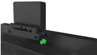
Gently press the NFC Reader into the peripheral bay making sure the connector is mated.
