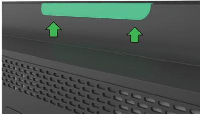
Remove the selected peripheral cover from the display head to expose the peripheral bay.
