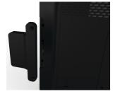
Gently press the fingerprint reader into the peripheral bay making sure the connector is mated.
