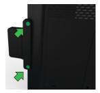
Remove the protective film from the included mylar covers and place the covers over the screws.
